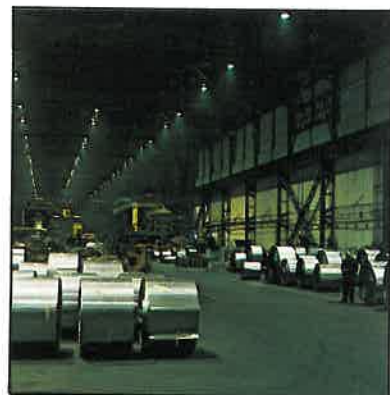
Above Steel rolling mills at Trostre, Wales, lit by high bay discharge lamps. Top Left Spectacular scene a mile inside a north Wales mountain, illuminated by SONline high pressure sodium floodlights. The excavations are for the CEB's Dinorwic pumped storage power station at Llanberis. Left Section of motorway near Coventry illuminated by low pressure sodium lamps.
