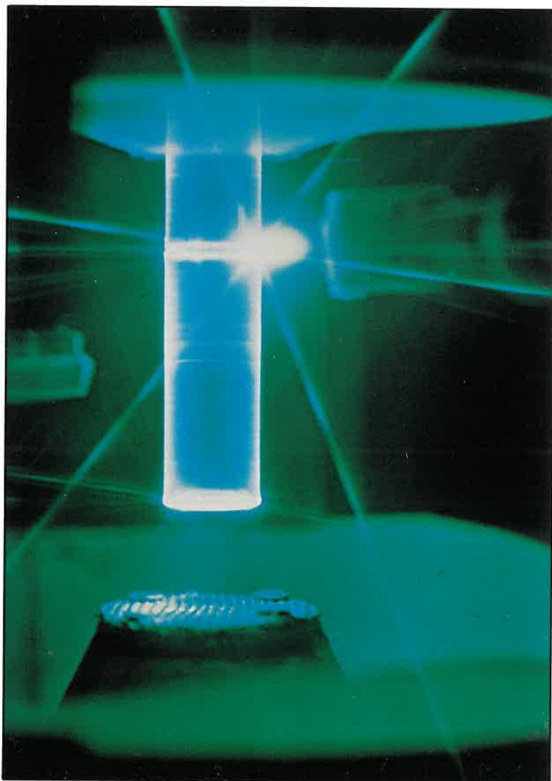
Right Latest technology; a powerful industrial laser is used to cut quartz during production of tungsten halogen lamps.
