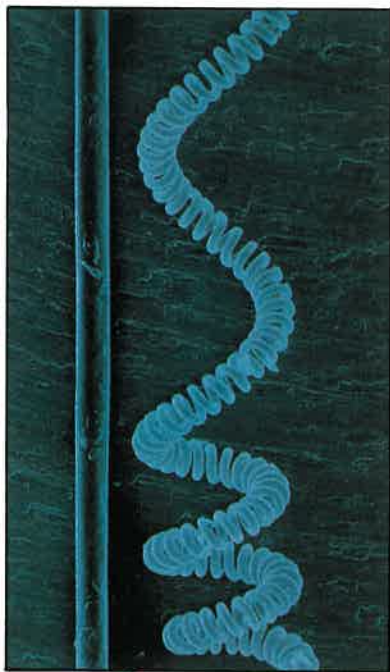
Above Modern filaments are made of tungsten, a material which can withstand extremely high temperatures. So that they can be heated to incandescence quickly with a minimum amount of current they are made extremely fine – far finer than a human hair, as this picture shows.
